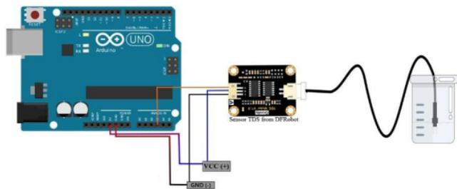
Gambar 6 Rangkaian kalibrasi sensor TDS.
