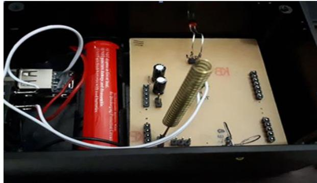
Gambar 8. *Sensor Radar Microwave*
