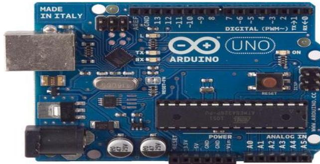
Gambar 1. Board Arduino Uno
