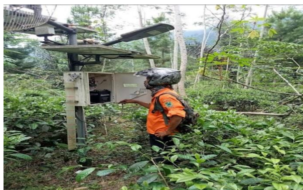
Picture 7. Checking and Maintenance of Early Warning System (EWS) tools by BPBD Banjarnegara and Disaster Resilient Village Volunteers Sirongge Village
