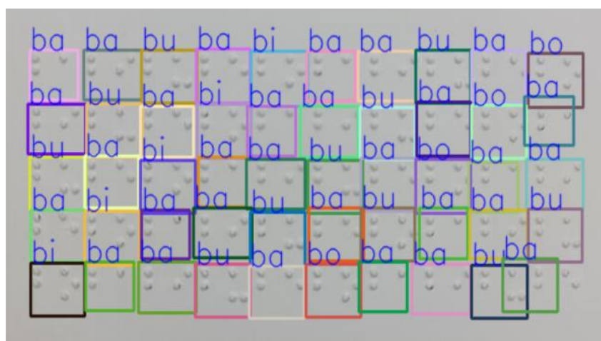
Figure 13. Qualitative examples of Braille cell detection and syllable-level classification results produced by the proposed Faster R-CNN framework.
