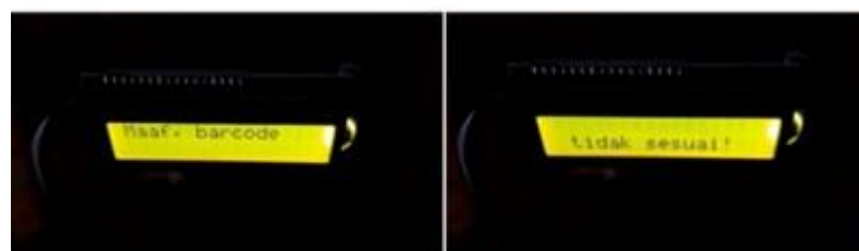
LCD message if the barcode does not match/is not registered in the database. "Sorry, barcode does not match"
